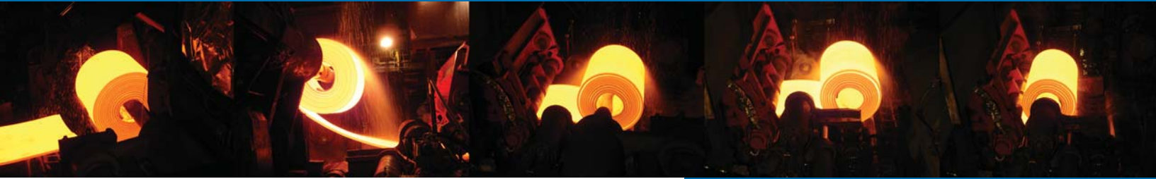
Hybrid-Mandrelless Coilbox™ operation
