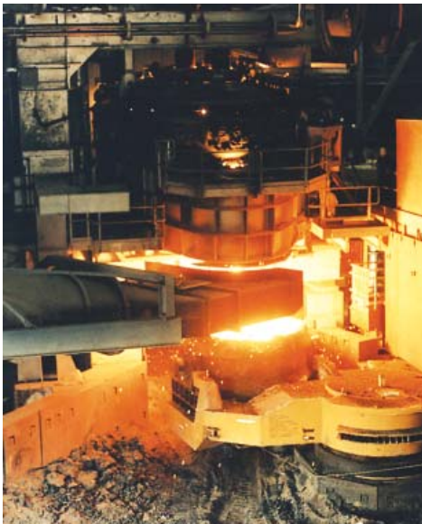
Tapping operation with newly developed fume collection system
