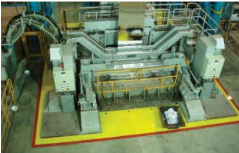
Hatch Coating Mass Control System (CMC) is an operator and maintenance-friendly system designed collaboratively by engineers and operators
