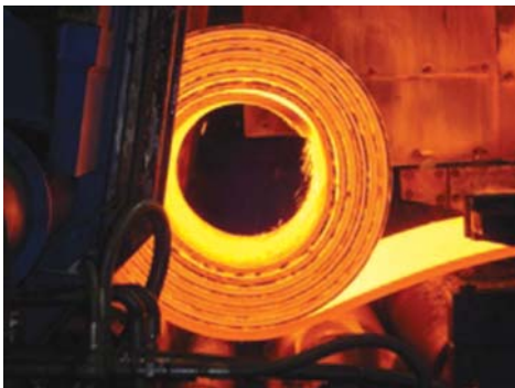
Coilbox™ technology developed and commercialized by Hatch Technologies – a technology expert in the global community for hot strip mills
