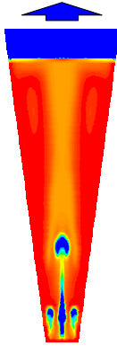
CFD Model based volume fraction prediction of liquid-solid fluid bed reactor (red = solids, blue = liquid)
