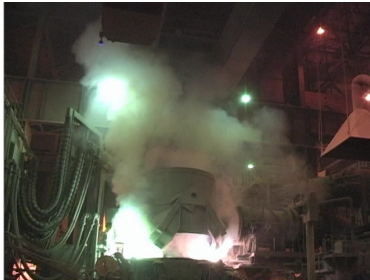
Typical fume burst emitted during scrap charging of an EAF.
